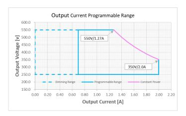
**Note:** EUCO ARENA SPORT 2K1 series can be programmed with wide output current through computer and programming tool. For more details, please refer to DALI programming User Manual or RDM/DMX programming User Manual.
